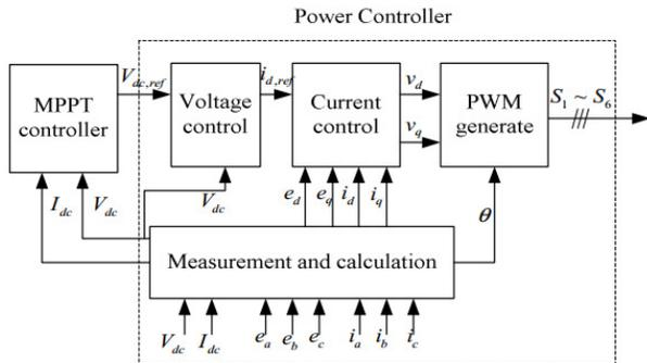
Fig.5. The control system diagram of SSGCPS
