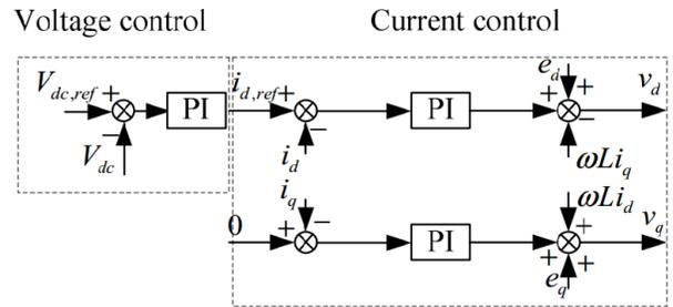
Fig.7. The voltage control and current control unit
