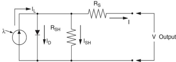
Fig.2 Equivalent circuit of PV module showing the diode and ground leakage currents
