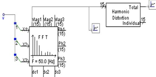
Figure.11. FFT and THD Blocks in PSCAD
