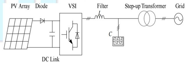
Fig.1. A typical configuration of a three phase SSGCPS
