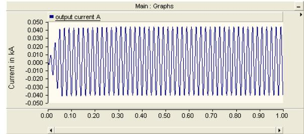
Figure.12. Output Current waveform for Phase A
