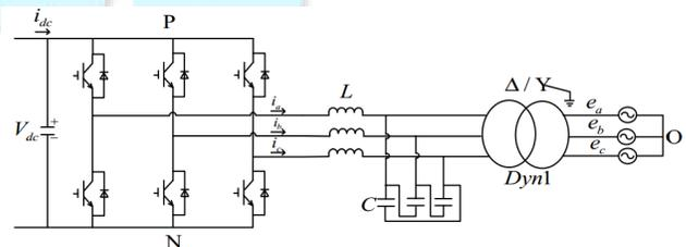
Fig.4. The electrical configuration of PV inverter for grid connection
