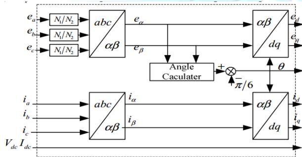
Fig.6. The measurement and calculation unit
