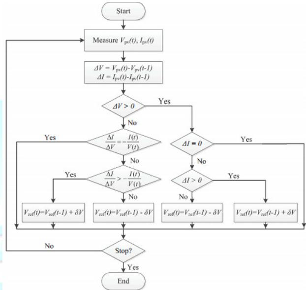
Fig.3. The flow diagram of MPPT
