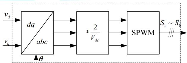
Fig.8. The PWM generate unit
